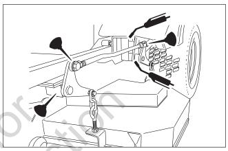
Figure 20. Deck Lift Linkage Pivots
